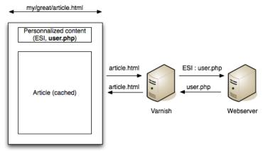
Edge Side Includes or ESI is a small markup language for dynamic web content assembly at the reverse proxy level. The reverse proxy analyses the HTML code, parses ESI specific markup and assembles the final result before flushing it to the client.
