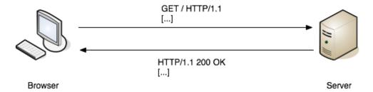
The client sends an HTTP request to the server which returns an HTTP response with the message body.
